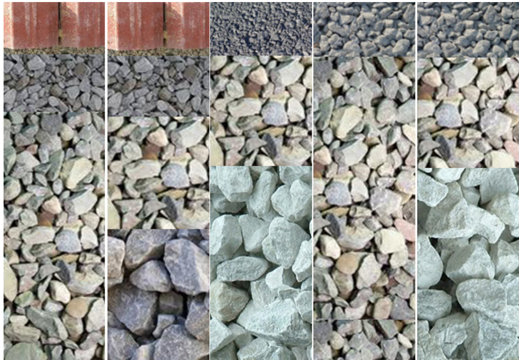
Figure 2.11.11 Commonly used stone for choker and reservoir layers (not to scale).
