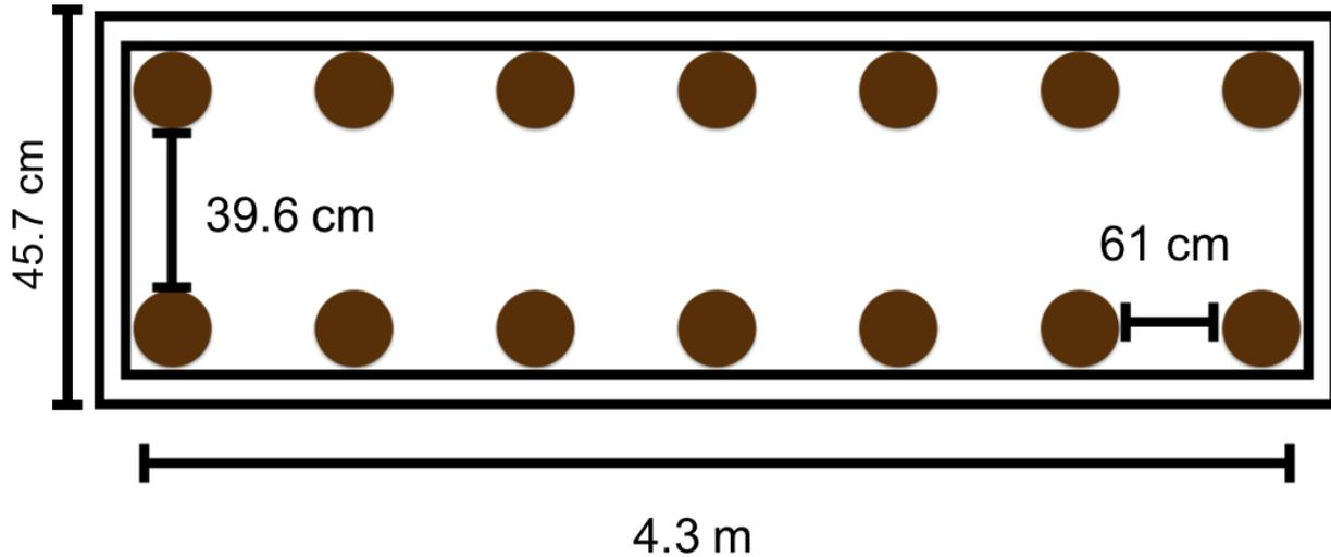
*Figure 6: Diagram of a breakwall*
